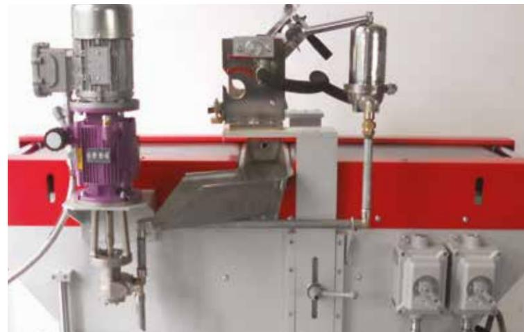
**Curtain coaters:** K2 variator on a dosing pump (Atex ambient)
